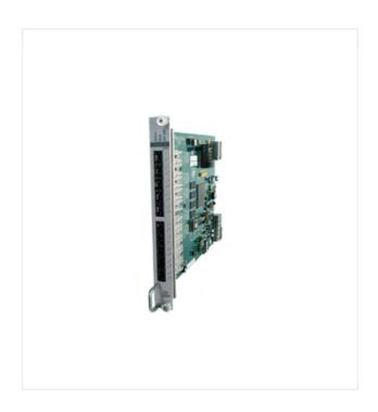
ports on the card can be used to support fiber services to 20 customers per card. The card also supports single channel SFP's for a total of 10 subscribers per card.
