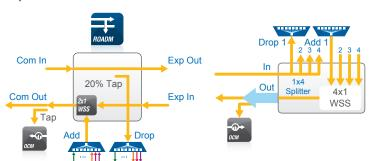
In addition to local add and drop capabilities, ROADMs provide channel pass-through capabilities that enable optical mesh networks and extend their reach. This minimizes the need to terminate wavelengths at each site and reduces the quantity of transponders in the network, thereby lowering equipment and operational costs.
