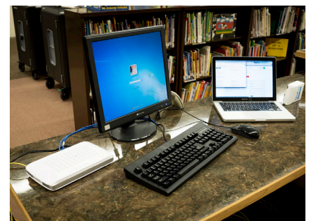
An Optical Network Terminal (ONT) provides Internet services to all of the devices on the librarian’s desk.
